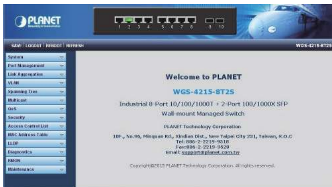
Figure 5-3: Web Main Screen of Wall-mount Managed Switch
